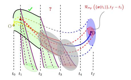
Compute minimum volume outer ellipsoids: SDP
